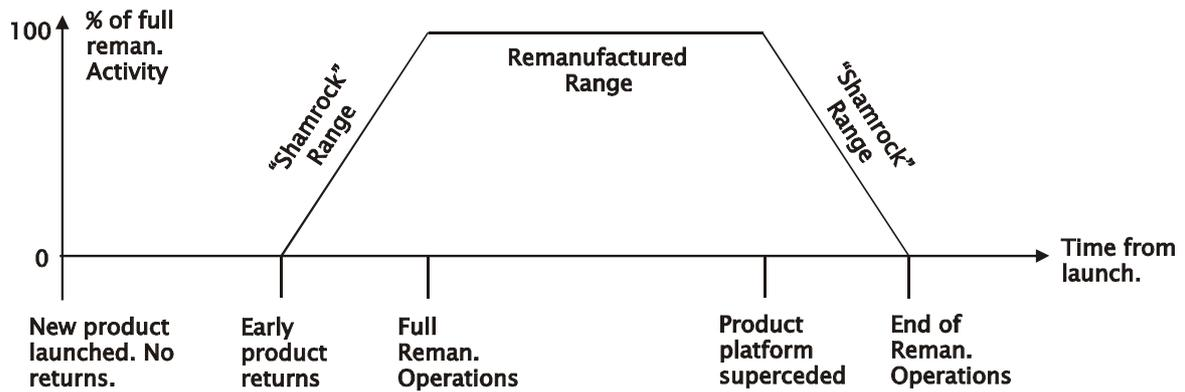
Figure 5: The Xerox Remanufacturing Ramp Up/Down for each Product Line
