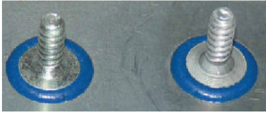
Figure 1: Commercial aluminum inserts (head diameter 12mm, Raybond™) bonded to aluminum car body sheet with epoxy adhesive
