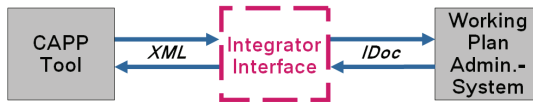
Figure 7. Working plan transfer from the production process planning tools to the working plan administrative system (and backwards)
