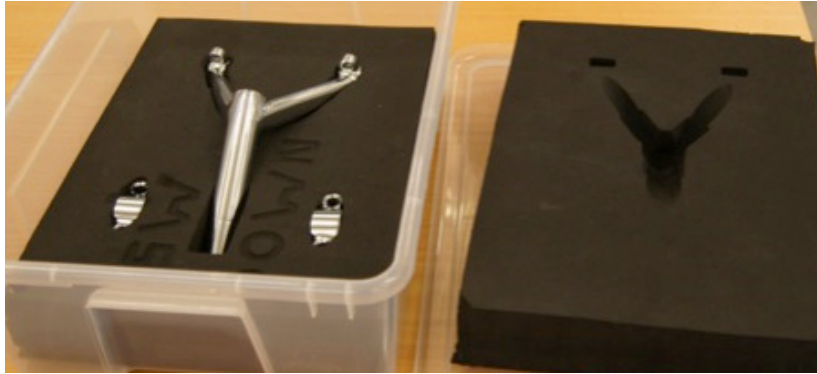
Figure 8. Finished example packaging manufactured from neoprene foam
