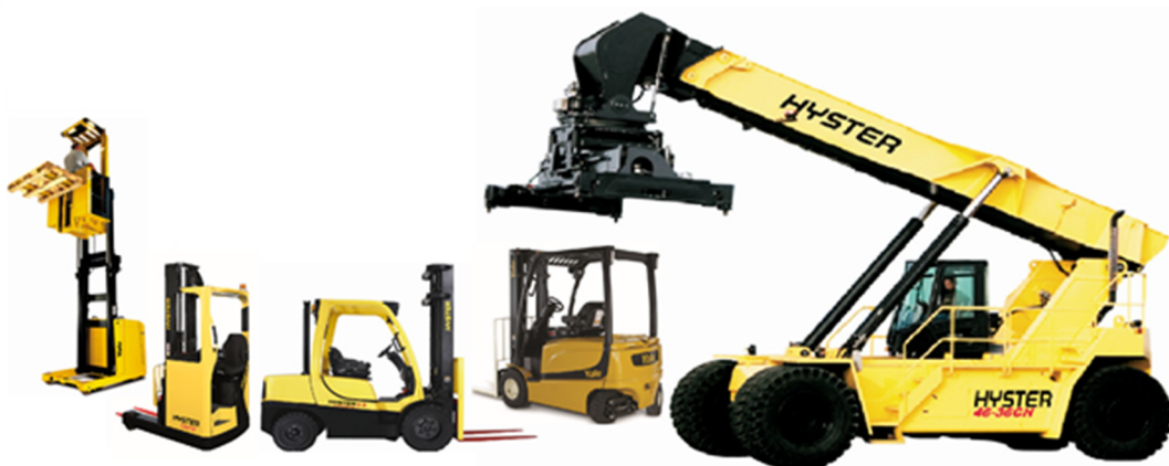
Figure 2. Left to right: VNA truck, reach truck, ICE counterbalanced, Electric counterbalanced, reach stacker
